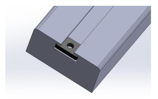
• Fit the platform rack & WR04 brackets onto the cross bars and fix into place using the fittings & key ways.
