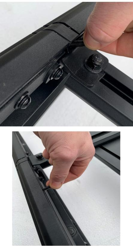
• Slide T-slot bolts within the recessed channel to be roughly in position where mounting brackets will fix. This is – 4 T-slots per side – 2 towards the front on either side and 2 towards the rear on either side.
