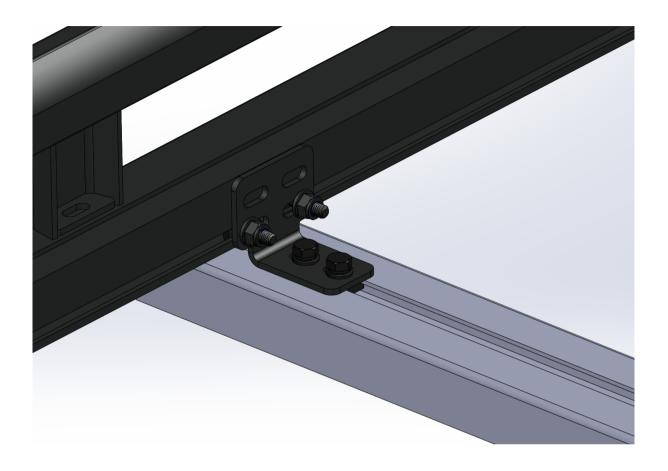
• Re fit rubber sealing strip and tighten all fittings once platform rack and cross bars are in their desired position.
